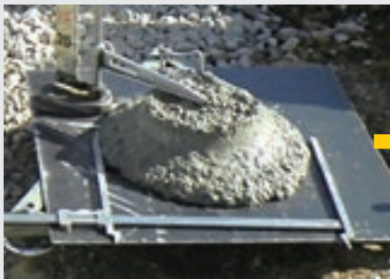
⑥ Regular concrete (Slump flow 37cm)
