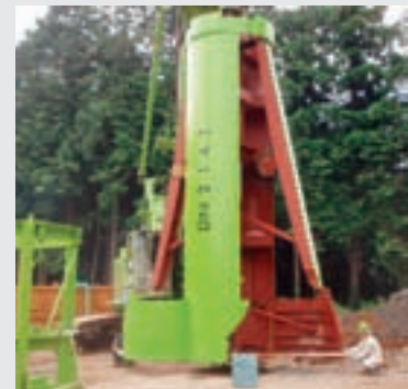
② New OMR/B excavator (shaft diameter=2,100mm, belling diameter=4,700mm)
